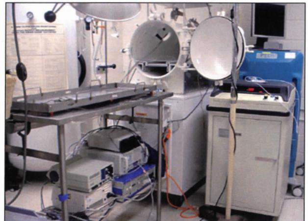
Figure 2. Customized hyperbaric laboratory used to study decompression sickness at VCURES.
