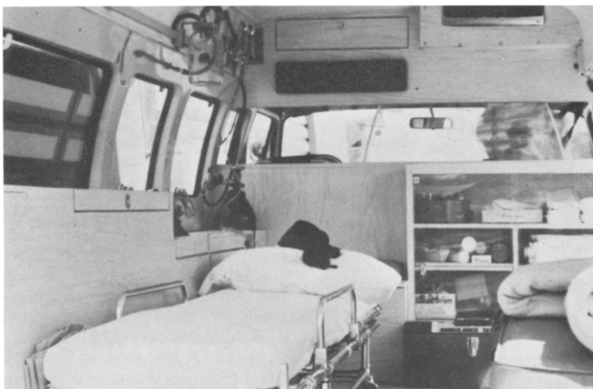
Figure 2. Interior of ambulance. Note high headroom and overall spaciousness.
