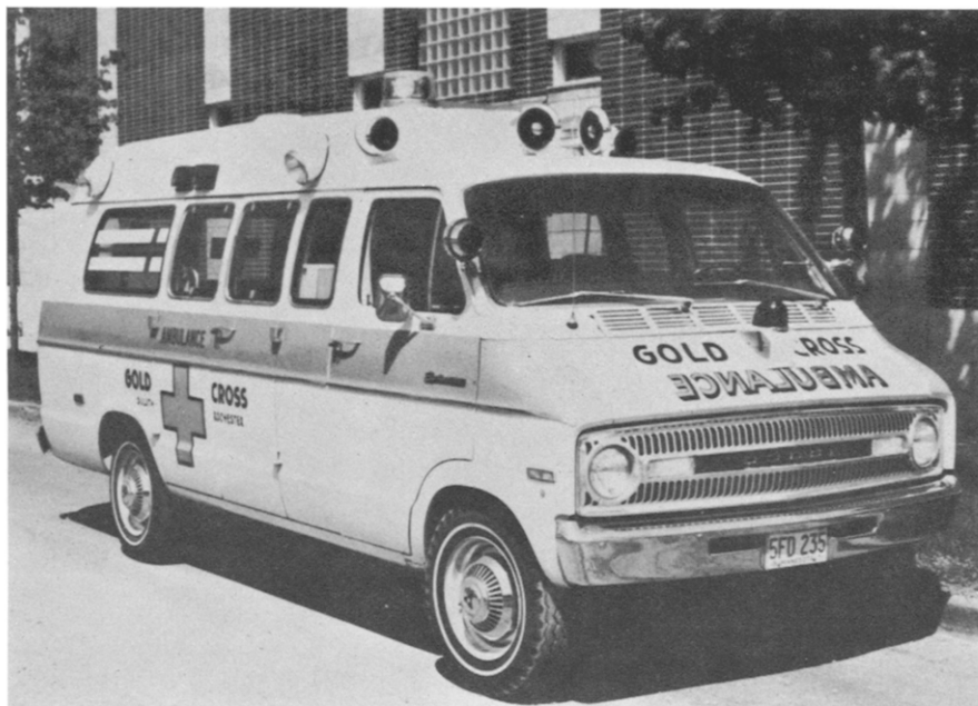
Figure 1. Van type of ambulance. Mirror-image lettering of AMBULANCE facilitates identification of approaching vehicle via rear-view mirror.
